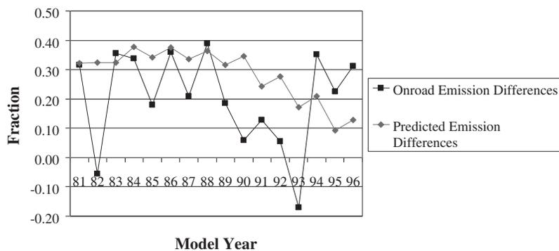
Figure 9: Carbon Monoxide (CO) Differences in Inspected and Uninspected Trucks
