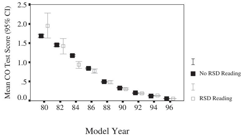
**Figure 6: Inspection/Maintenance (I/M) Test Scores for Carbon Monoxide (CO): Vehicles With and Without On-Road Remote Sensing Devices (RSD) Reading**
