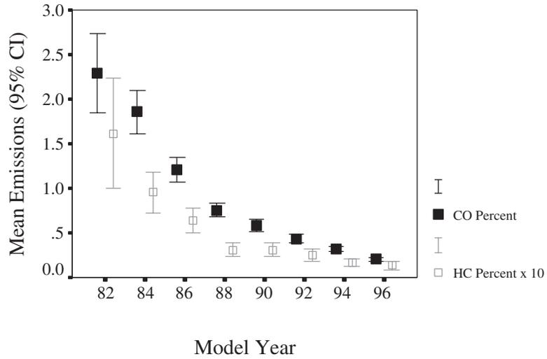
**Figure 1: On-Road Carbon Monoxide (CO) and Hydrocarbons (HC), by Model Year**
