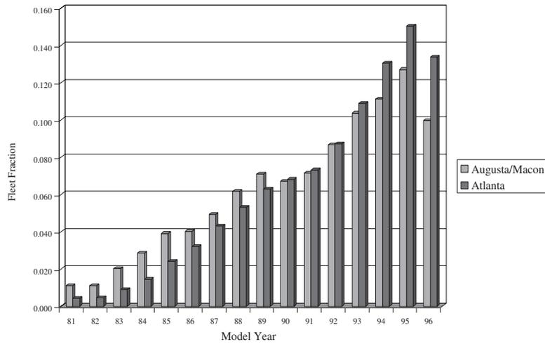
**Figure 2: On-Road Model Year Comparison: Inspection/Maintenance (I/M) (Atlanta) Versus Non-I/M (Augusta-Macon) Vehicle Fleets**
